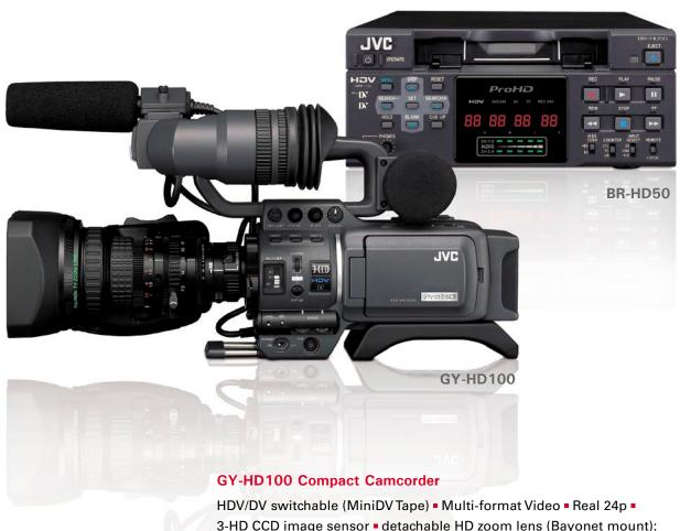
HDV/DV switchable (MiniDV Tape) • Multi-format Video • Real 24p • 3-HD CCD image sensor • detachable HD zoom lens (Bayonet mount): zoom/focus/iris mechanical control • Magnesium die cast body • Detachable professional Viewfinder • TC capability • External HDD capability • Set-up with SD memory card
